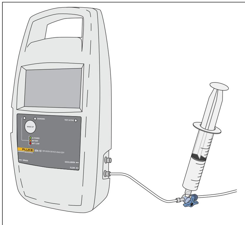
Figure 3. Infusion Device Connections to the Product
