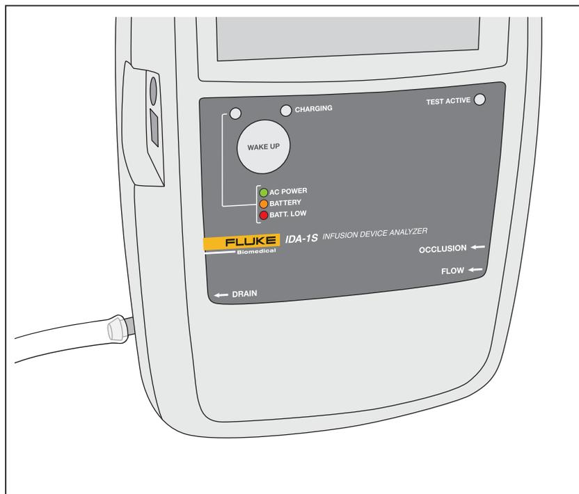
**Figure 4. Drain Connections to the Product**
